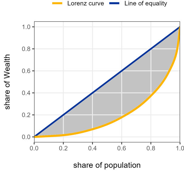
Figure 1: Lorenz curve for a Pareto distribution. The shaded area is called the area of concentration.
